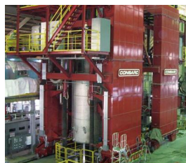
150トン電極スラグ溶解炉 150-ton Electroslag Remelting Furnace
