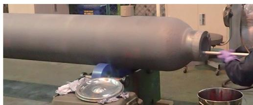
Procedure of Penetrant Test
